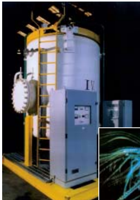
Reaction vessel, metering and monitoring equipment for treatment of 3,600m 3 /hr sea water offshore Brazil
