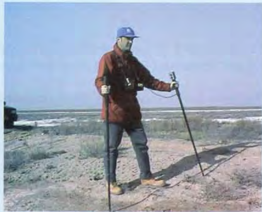
DCVG Survey on a pipeline in Eastern Europe
